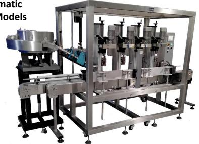
The ROPP Capping Machine is built to thread aluminum roll-on pilfer proof (ROPP) caps onto containers. Aluminum blanks are threaded using custom capping heads for the closure employed on any given packaging project. Common in the wine and distilled spirits industry, these cappers are gaining popularity in other industries that desire tamper evident sealing for their products.
